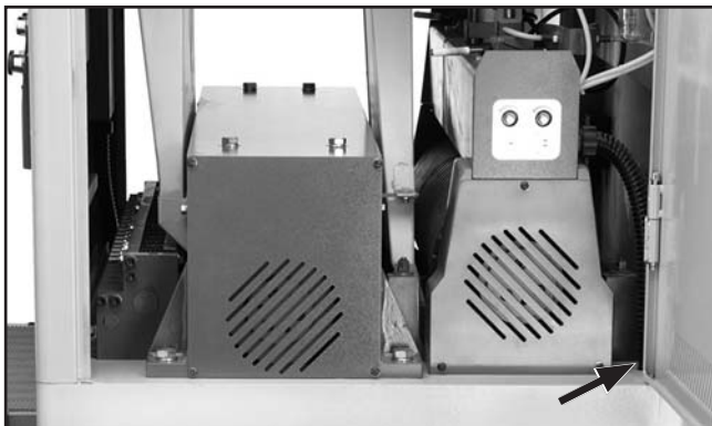
Figure 60. Right rear table-frame height check location.
